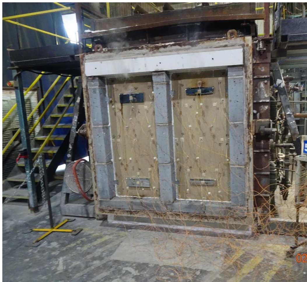
The unexposed face of the doorsets after a test duration of 40 minutes
