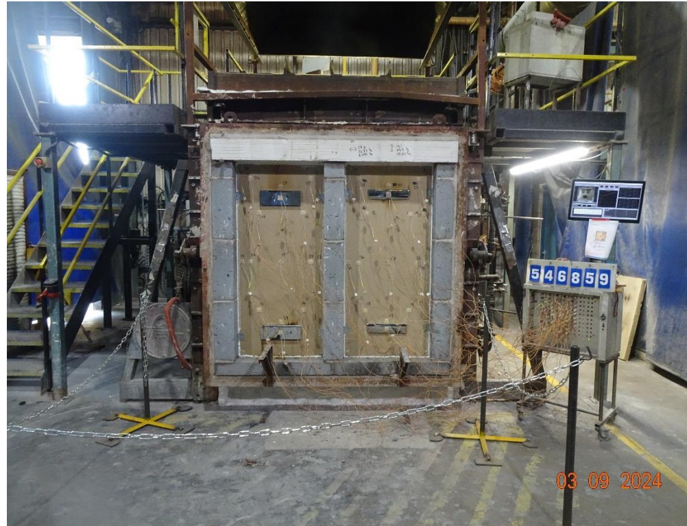
The unexposed face of the doorsets after a test duration of 20 minutes
