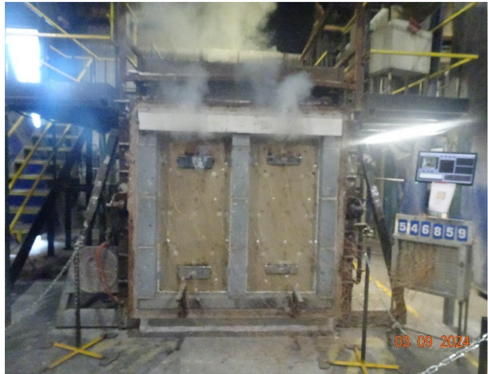
The unexposed face of the doorsets after a test duration of 60 minutes
