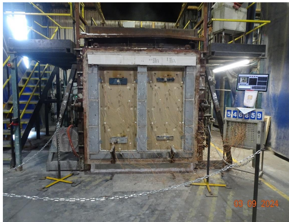
The unexposed face of the doorsets after a test duration of 40 minutes
