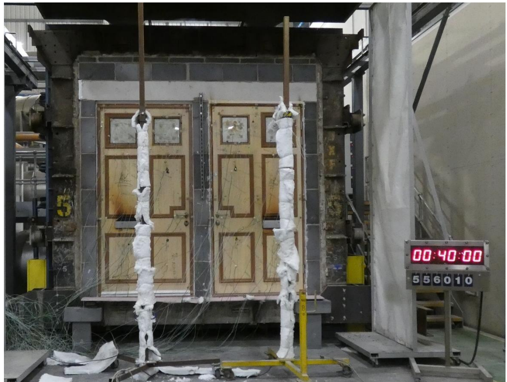
The unexposed face of the specimens after a test duration of 40 minutes
