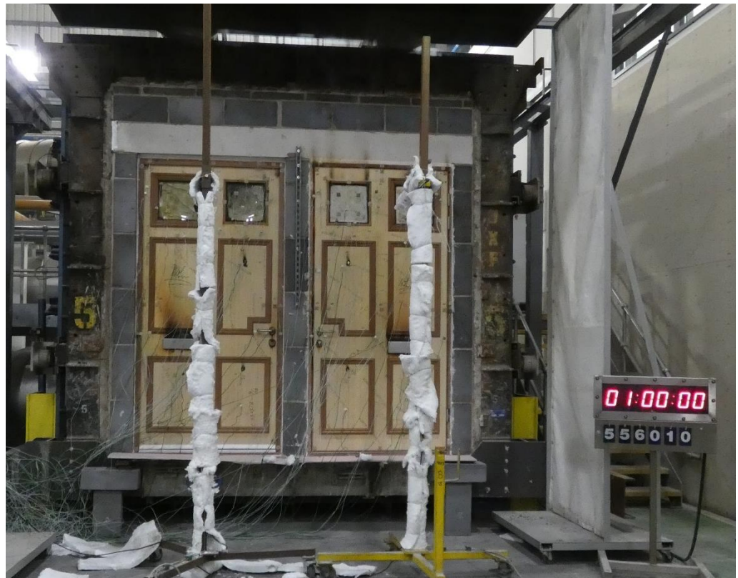
The unexposed face of the specimens after a test duration of 60 minutes
