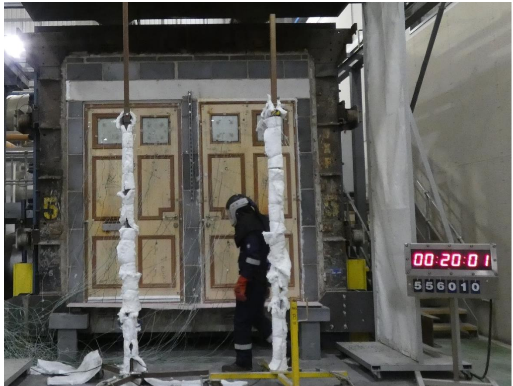
The unexposed face of the specimens after a test duration of 20 minutes
