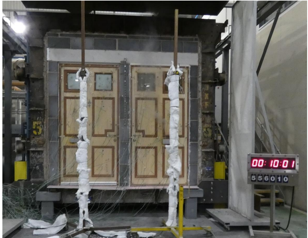
The unexposed face of the specimens after a test duration of 20 minutes
