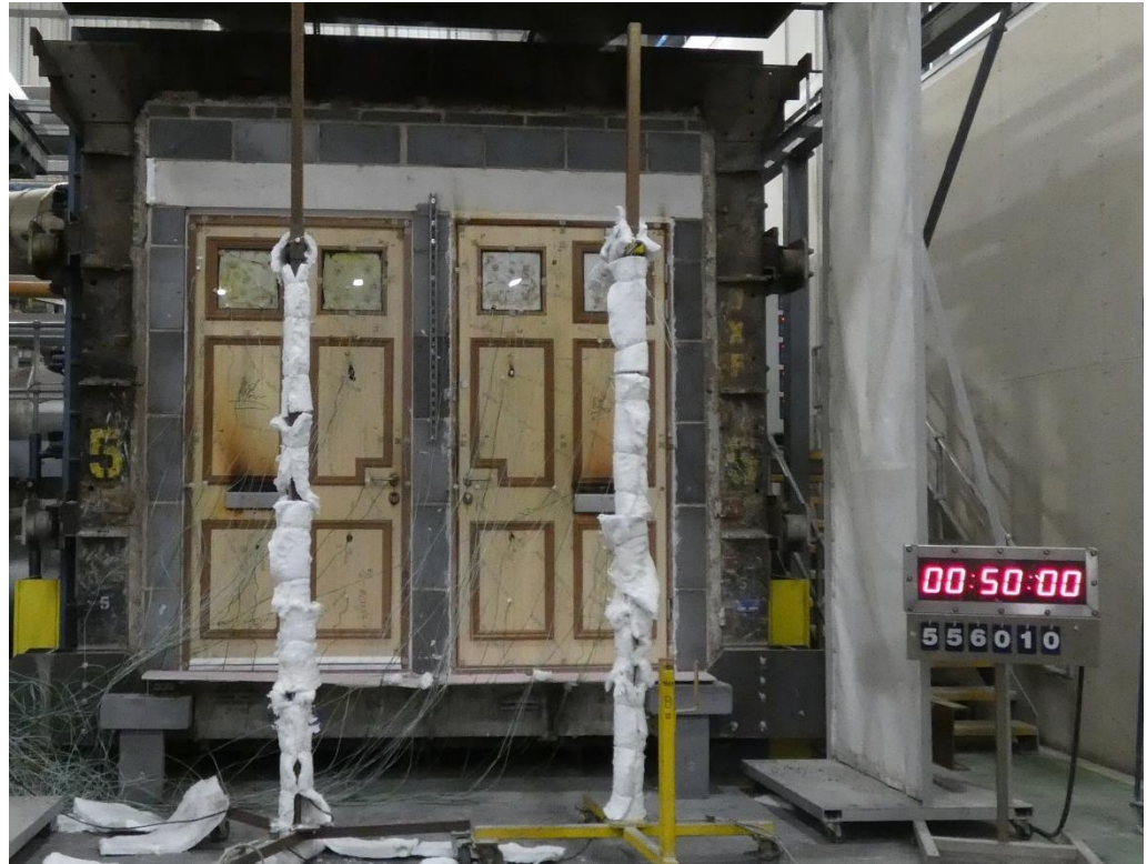
The unexposed face of the specimens after a test duration of 50 minutes
