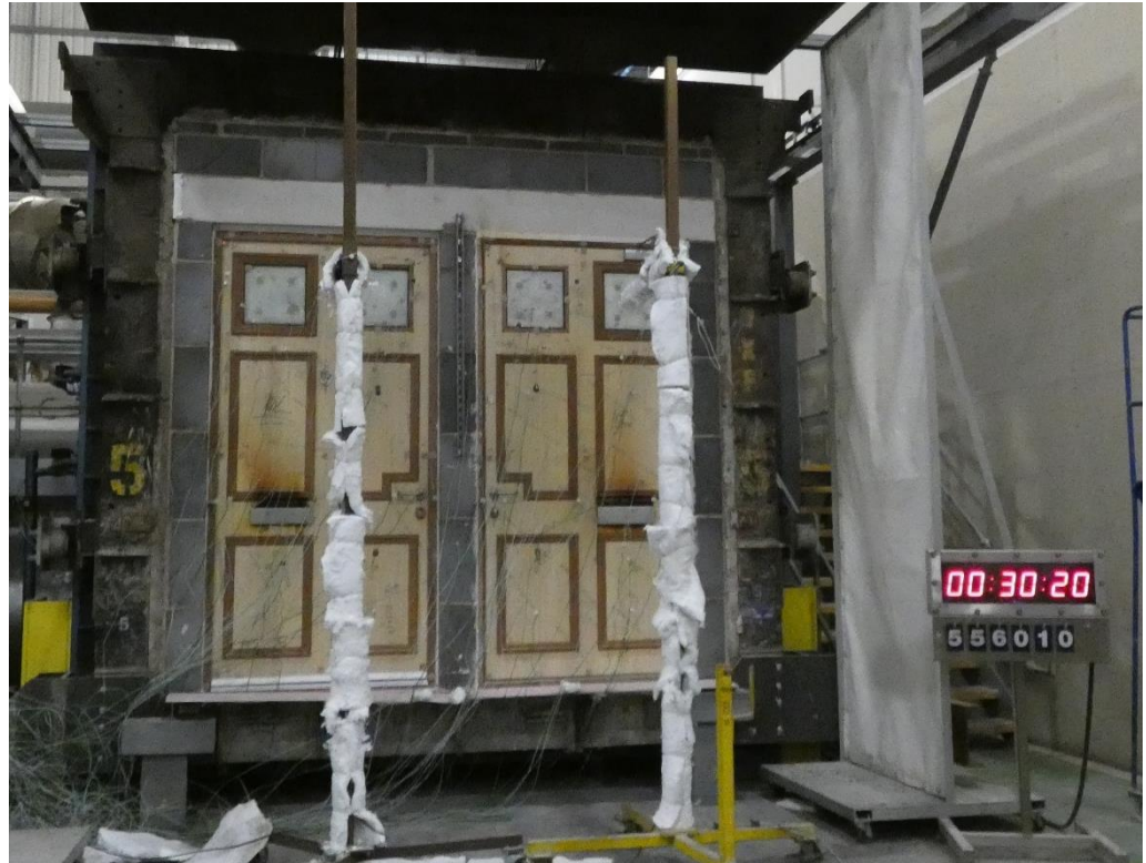
The unexposed face of the specimens after a test duration of 30 minutes
