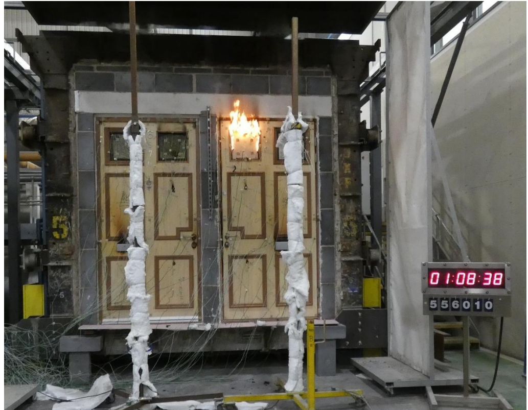
The unexposed face of the specimens after a test duration of 68 minutes showing sustained flaming on Doorset B
