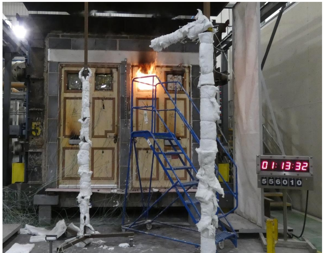
The unexposed face of the specimens after a test duration of 73 minutes
