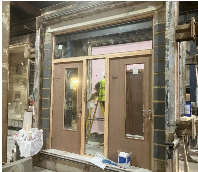
Figure 30 Unexposed face of the specimen before the start of the test
