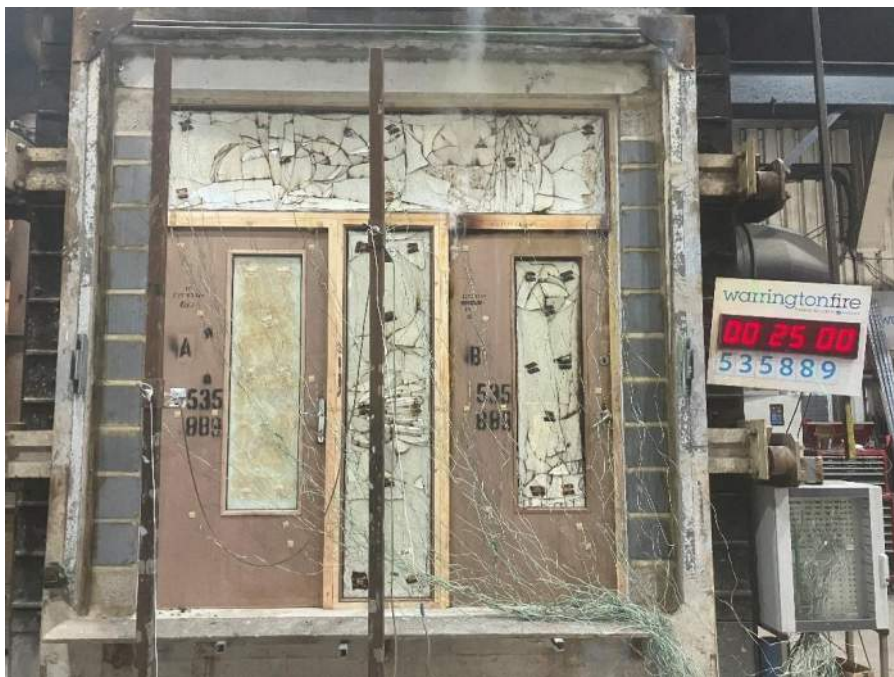
Figure 35 Unexposed face of the specimen after 25 minutes of testing
