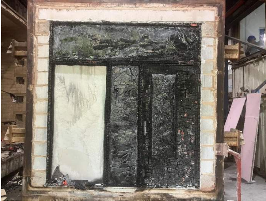
Figure 38 Exposed face of the specimen at the end of the test
