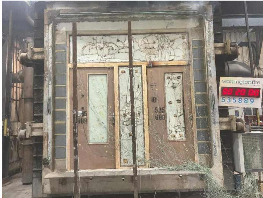
Figure 34 Unexposed face of the specimen after 20 minutes of testing
