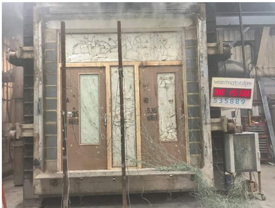
Figure 33 Unexposed face of the specimen after 15 minutes of testing
