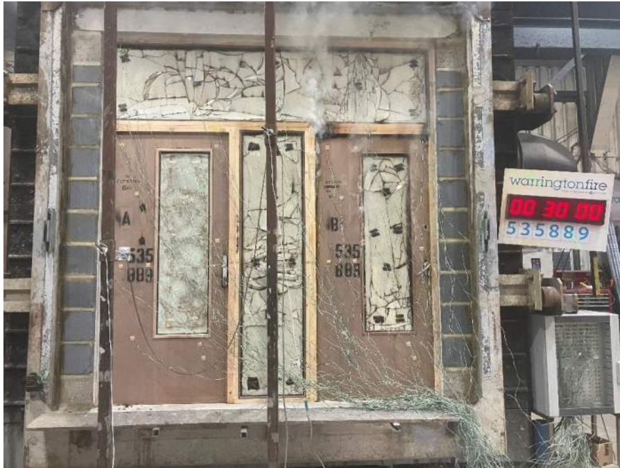
Figure 36 Unexposed face of the specimen after 30 minutes of testing
