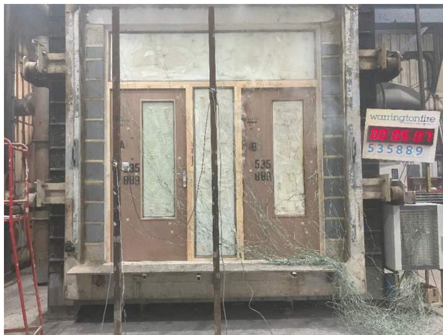
Figure 31 Unexposed face of the specimen after 5:07 minutes of testing
