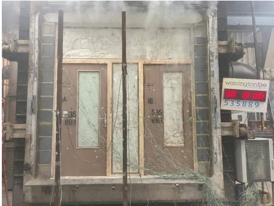
Figure 32 Unexposed face of the specimen after 10 minutes of testing
