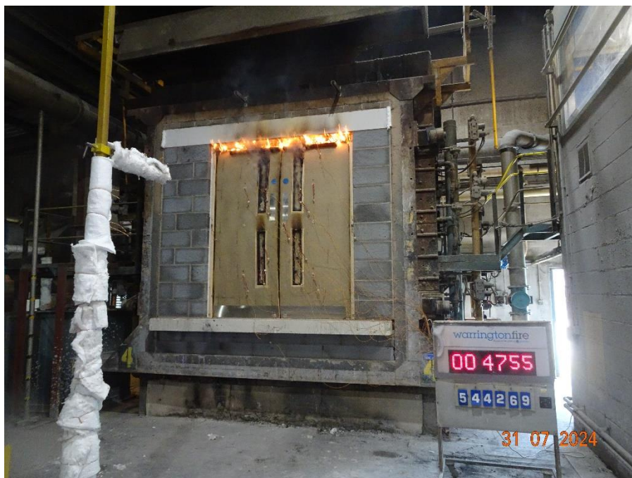
Figure 28 Unexposed face of the specimen at 47 minutes 55 minutes of testing displaying sustained flaming before the test was discontinued
