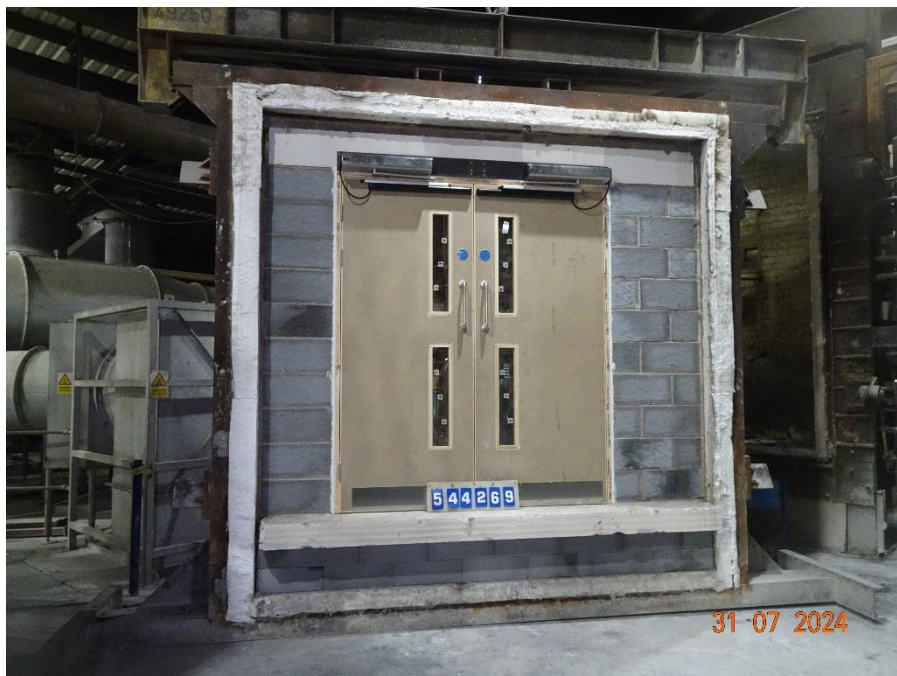
Figure 24 Exposed face of the specimen before the start of the test
