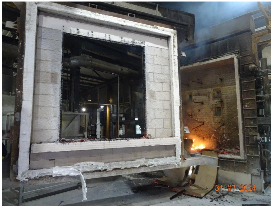
Figure 29 Exposed face of the specimen at the end of the test
