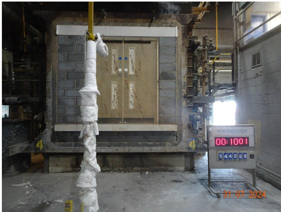
Figure 25 Unexposed face of the specimen at 10 minutes of testing
