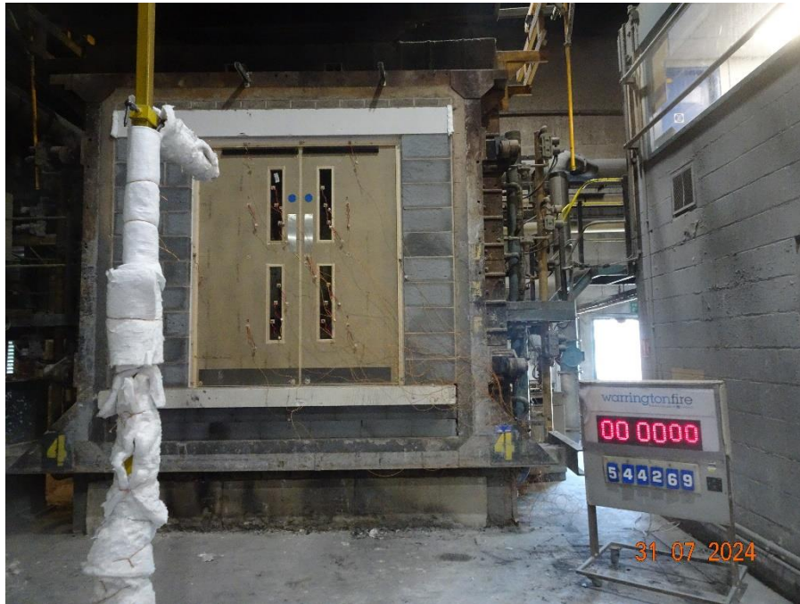
Figure 23 Unexposed face of the specimen before the start of the test
