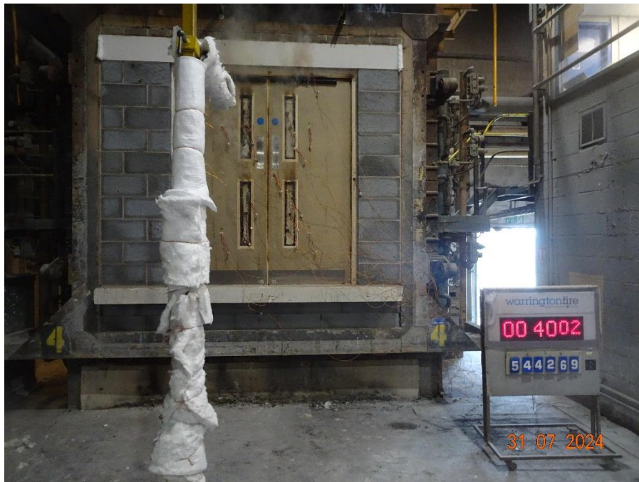
Figure 27 Unexposed face of the specimen at 40 minutes of testing
